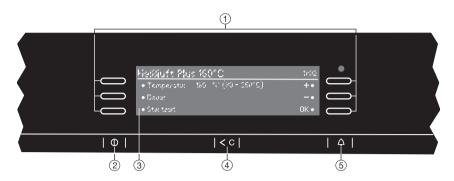
The appliance is operated via the display ③ and the electronic sensors next to and below the display. These react to finger contact. A keypad tone will sound each time a sensor is touched. The volume of the keypad tone can be adjusted or switched off altogether (see "Settings - Volume").
